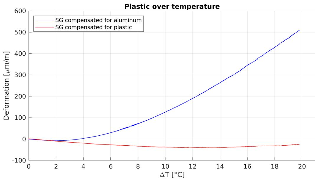
(b) Deformation dependence over temperature difference
