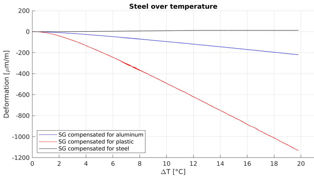
(b) Deformation dependence over temperature difference
